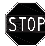
30" x 30" WHITE ON RED REFLECTORIZED 7'-0" MOUNTING HEIGHT (R1-1)
