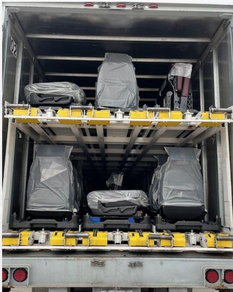
Auto-loaded packaged seat sets to customer (front, middle, and rear seat sets)
