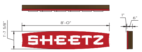
canopy mounted sheetz sign detail SCALE: 1/2" = 1'-0"
