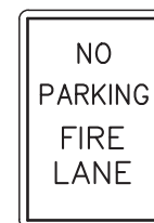
12" x 18" RED ON WHITE REFLECTORIZED 7'-0" MOUNTING HEIGHT (UR7-22)
