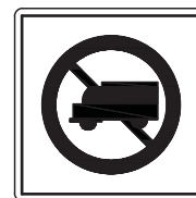
24" x 24" RED & BLACK ON WHITE REFLECTORIZED 7'-0" MOUNTING HEIGHT (R5-2)
