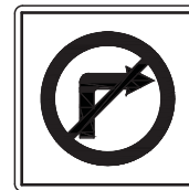
24" x 24" RED & BLACK ON WHITE REFLECTORIZED 7'-0" MOUNTING HEIGHT (R3-1)
