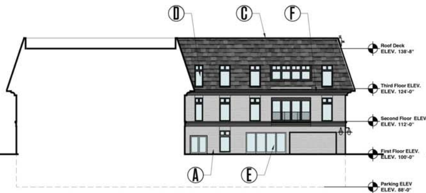
2 West Elevation SCALE: 1/16" = 1'
