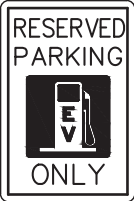
12" x 18" GREEN TEXT WITH BLUE SYMBOL ON WHITE REFLECTORIZED 7'-0" MOUNTING HEIGHT ELECTRIC VEHICLE PARKING SIGN DETAIL NOT TO SCALE
