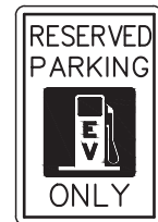
12" x 18" GREEN TEXT WITH BLUE SYMBOL ON WHITE REFLECTORIZED 7'-0" MOUNTING HEIGHT ELECTRIC VEHICLE PARKING SIGN DETAIL NOT TO SCALE
