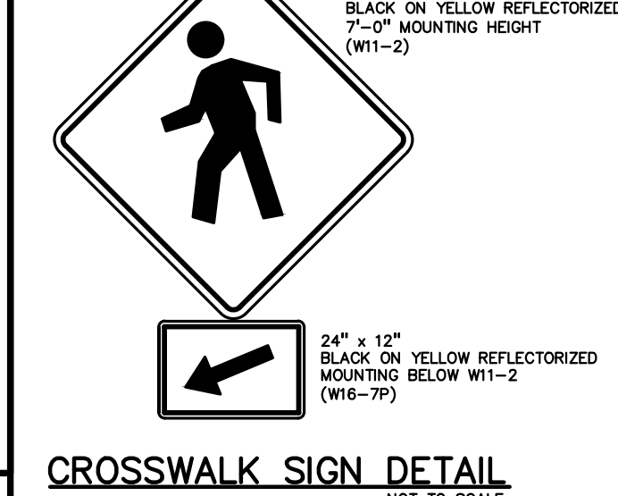
CROSSWALK SIGN DETAIL NOT TO SCALE
