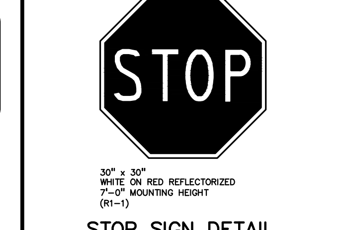
STOP SIGN DETAIL NOT TO SCALE
